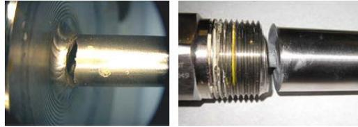
So it is necessary to establish if the resulting dynamic tensions are lower than those supported by the material maximum fatigue limit. If they are not, replace the thermowell installing one whose dimensions can support the current dynamic stress.
